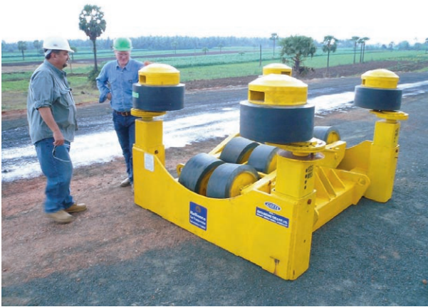
Figure 4. Launching roller 80 t.
